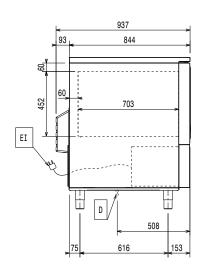
Drain Electrical inlet (power)
